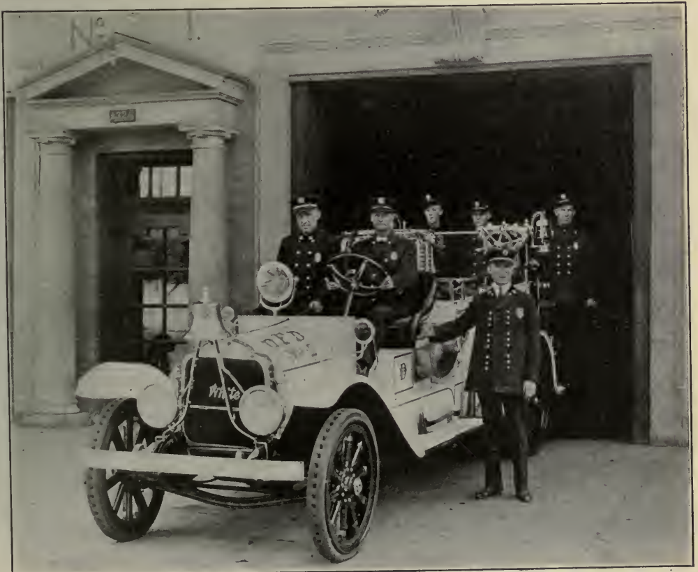
A WHITE COMBINATION HOSE AND CHEMICAL FIRE TRUCK IN SERVICE IN DENVER, COLO.
